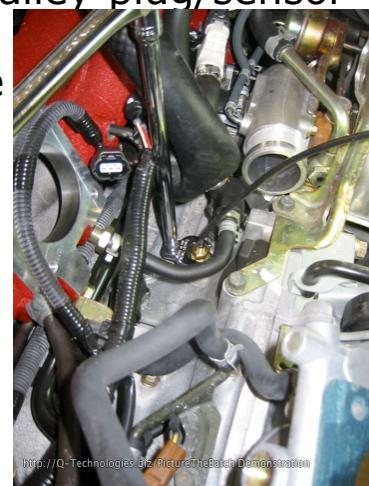
12. Reinstall throttle body. The service manual recommends that you use a new throttle body gasket. Your stock gasket will most likely still be in new condition, but do keep in mind that it might also not be. Be prepared. Tighten to 5.8 ft-lbs or 8 Nm
