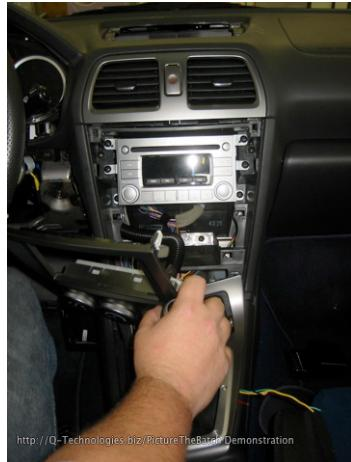
the removal of two screws that hold the bottom end of the cover. After these have been removed, pry the cover from the bottom up.
