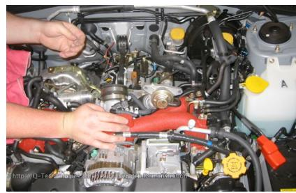
3. Remove throttle body. Start by removing the two wire harnesses from the unit. Then use a 10-mm socket to remove all four bolts.
