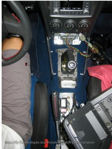
Remove the screws (2) in the lower part of the front of this piece. There are 4 tabs holding this section to the side/front pieces, pry these out.
