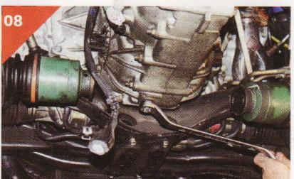
BEFORE WE GET TOO FAR INTO THE TEARDOWN, DRAIN THE TRANSMISSION FLUID BEFORE ATTEMPTING TO YANK OFF THE DRIVESHAFT. WE NOTICED THE MAGNETIC DRAIN PLUG HAD UNWANTED METAL SHAVINGS. LOOKS LIKE A TRANNSY REBUILD WITH SOME STRAIGHT CUT GEARS OR HELICAL TYPE IS COMING UP FASTER THAN WE EXPECTED.
