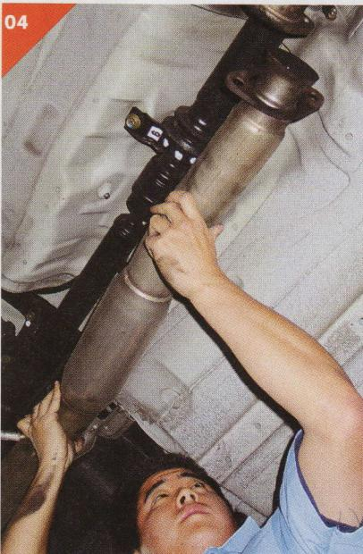
WITH THE DOWNPIPE OUT OF THE WAY, REMOVE THE EXHAUST SYSTEM. YOU DON'T NECESSARILY HAVE TO TAKE THE WHOLE UNIT OFF. JUST REMOVE THE B-PIPE WHILE YOUR CANISTER CAN REMAIN INTACT.
