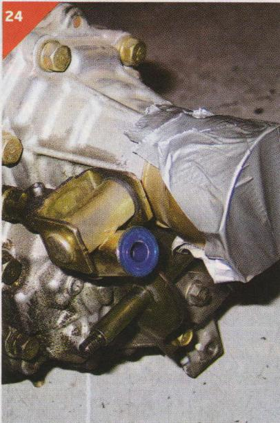
IT'S IMPORTANT TO ALWAYS PROTECT THE INTERNALS OF THE OIL SEAL FROM CONTAMINANTS ONCE THE TRANNY WAS REMOVED.
