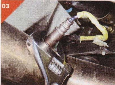
UNBOLT THE AFTERMARKET OR FACTORY DOWNPIPE WITH THE HELP OF SOME WD40 IF YOUR NUTS AND BOLTS ARE FROZEN ONTO PLACE WITH RUST. USE A CRESCENT WRENCH TO EASILY REMOVE THE O2 SENSOR. GO AHEAD AND JUST LEAVE IT HANGING FOR THE TIME BEING. THE UNIT WILL COME OFF WITH THE TRANNSY BRACKET LATER.
