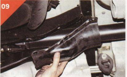
UNBOLT THE SIX BOLTS HOLDING UP THE DRIVESHAFT PROTECTOR.
