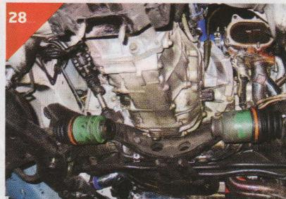
ONCE THE TRANNY HAS BEEN PROPERLY ALIGNED, REINSTALL THE BELL HOUSING BOLTS AND TWO NUTS TO THE SUBARU SUGGESTED TORQUE OF 36.9 LB-FT.
