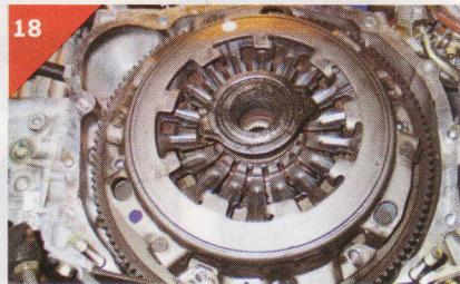
18 WHEN REMOVING THE FACTORY CLUTCH AND PRESSURE PLATE, REMEMBER TO ALWAYS REMOVE THE BOLTS IN A CROSS DIRECTIONAL STAR PATTERN TO PREVENT ANY WARPAGE TO THE UNIT.
