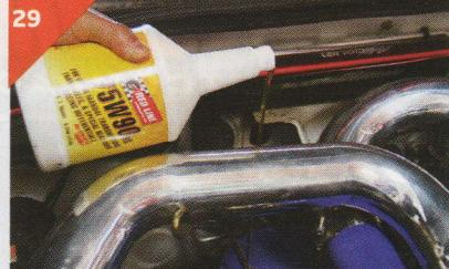
ONCE YOU HAVE COMPLETED THE INSTALLATION PROCESS AND DOUBLE CHECKED ALL BOLTS, USE THE TRANSMISSION FILLER DIP STICK AS A GUIDE FOR A FUNNEL TO REFILL THE TRANSMISSION. WE REFILLED THE SUBIE WITH 5.5 QUARTS OF 75W90 REDLINE FLUID. THE TRANSMISSION ITSELF TAKES 3.7 QUARTS WHILE THE FRONT DIFFERENTIAL CONSUMES 1.8 QUARTS. THEY ARE FILLED TOGETHER FROM THE SAME AREA.
