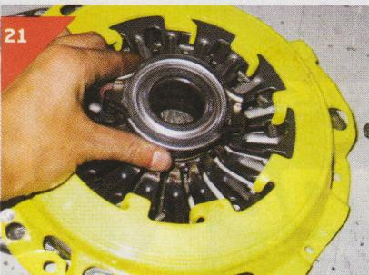
HERE'S AN IMAGE OF THE THROW OUT BEARING. DON'T INSTALL THE UNIT JUST YET. PUTTING IT ON NOW ONLY MAKES THE TRANSMISSION INSTALLMENT A LOT HARDER.
