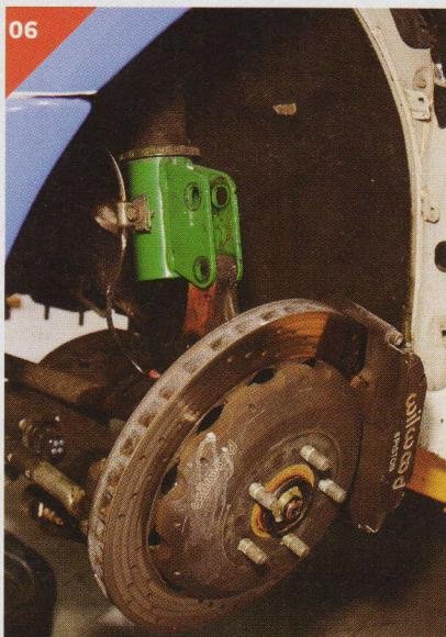
WITH BOTH FRONT TIRES OFF, UNBOLT BOTH FRONT STRUT TO HUB ASSEMBLY BOLTS IN PREPARATION TO REMOVE THE FRONT AXLES. PERFORMING THIS METHOD SAVES MORE TIME RATHER THAN THE TYPICAL SUBARU MANUAL DIRECTIONS REQUIRING SWAY BAR AND LOWER CONTROL ARM REMOVAL DISASSEMBLY.
