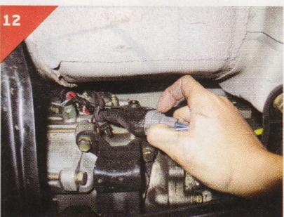
12 UNCLIP THE NEUTRAL SWITCH AND BACKUP SWITCH WIRES, MAKING SURE BOTH CLIPS AND WIRE LEADING TO THE ENGINE BAY HAVE BEEN FULLY DISCONNECTED. THE RUBBER SHIELDED O2 SENSOR CLIP ALSO NEEDS TO BE REMOVED. BE SURE, WHEN REMOVING THE TRANSMISSION, THAT ALL WIRES AND FOREIGN OBJECTS ARE CLEAR FROM BEING SNAGGED OR CAUGHT IN THE PATH OF THE TRANNY.
