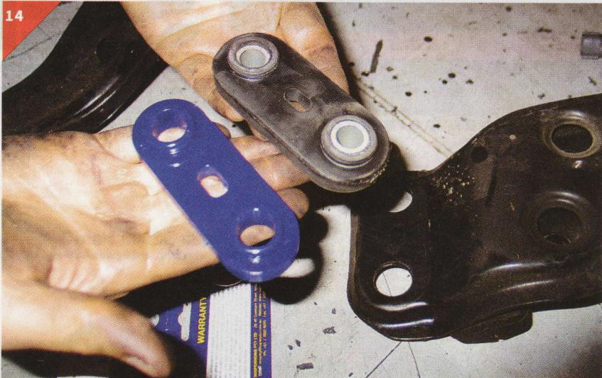
14 WE FIGURED NOW WAS AS GOOD OF A TIME AS EVER TO REPLACE THE FOUR FACTORY CUSHION RUBBERS WITH A SET OF SUPER PRO (FULCRUM PERFORMANCE) POLYURETHANE BUSHINGS. WE NOTICED WHEN GIVING THE VEHICLE A QUICK BLIP OF THE THROTTLE WHEN DRIVING, THE SHIFTER WOULD MOVE EXCESSIVELY DUE TO THE SOFT FACTORY BUSHINGS.
