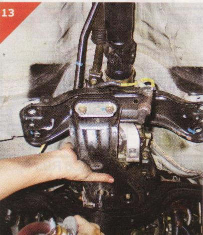
13 REMOVE THE SIX BOLTS HOLDING THE TRANSMISSION REAR CROSS MEMBER TO THE VEHICLE CHASSIS.
