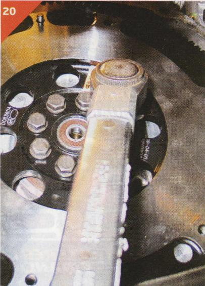
USE A RUBBER MALLET TO GENTLY TAP THE PILOT BEARING IN PLACE. USING A TORQUE WRENCH, INSTALL THE NEW ACT FLYWHEEL WITH A MIDWAY TORQUE OF 26.4 LB-FT ON ALL THE BOLTS BEFORE THE FINAL TORQUE SPEC.
