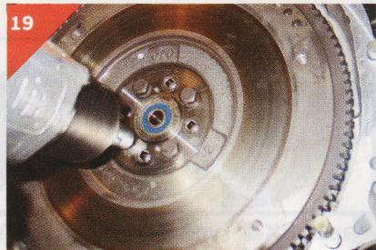
19 SUBARU SELLS A CRANKSHAFT STOPPER TO MAKE REMOVING THE FLYWHEEL EASIER. IF YOU LACK THAT CERTAIN PIECE OR JUST DON'T WANT TO BOTHER, HAVE A FRIEND OR YOUR MOM STAND IN THE FRONT OF THE VEHICLE HOLDING THE CRANK PULLEY WITH A BREAKER BAR WHILE YOU CRAWL UNDERNEATH AND REMOVE THE FLYWHEEL BOLTS IN AN ALTERNATING CRISS CROSS STAR PATTERN.
