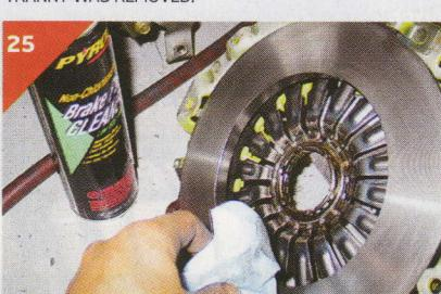
OIL OR SOLVENTS CAN RUIN A PERFECTLY GOOD CLUTCH WITH UNWANTED GLAZING. USE BRAKE CLEANER ON A CLEAN RAG TO WIPE OFF BOTH THE PRESSURE PLATE DISK AND FLYWHEEL TO CLEAN OFF ANY DEBRIS.
