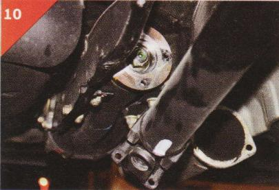
10 WHEN PREPARING TO REMOVE THE DRIVESHAFT, ASK A FRIEND TO JUMP IN YOUR SUBIE AND HOLD DOWN THE BRAKES FOR AN EASIER JOB REMOVING THE FOUR-BOLTS CONNECTING THE DRIVESHAFT TO THE AXLE HUB. THE TIGHT AREA LEAVES YOU WITH JUST ENOUGH ROOM TO USE AN OPEN-END WRENCH AND SOME BRUTE STRENGTH.
