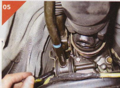
REMOVE THE GEAR SHIFT ROD (SHIFTER LINKAGE) AND STAY FROM THE TRANSMISSION. NOW WOULD BE A GOOD TIME IF YOU'RE LOOKING TO UPGRADE YOUR SHIFTER BUSHING FOR A FIRMER UNIT. THE FACTORY BUSHING GIVES THE WRX THAT SLOPPY FEELING WHEN SHIFTING OR IN GEAR.
