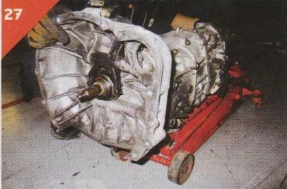
REINSTALLING THE TRANNY IS NEVER AN EASY TASK. WITH SOME HELP FROM YOUR FRIENDS HAVE SOMEONE MAKE SURE ALL THE WIRING AND HARD LINES ARE CLEAR OF THE TRANSMISSION'S PATH WHEN INSTALLING. IF YOU ARE USING A FLOOR JACK HAVE A FRIEND SLOWLY ELEVATE THE UNIT WHILE YOU GUIDE IT IN.
