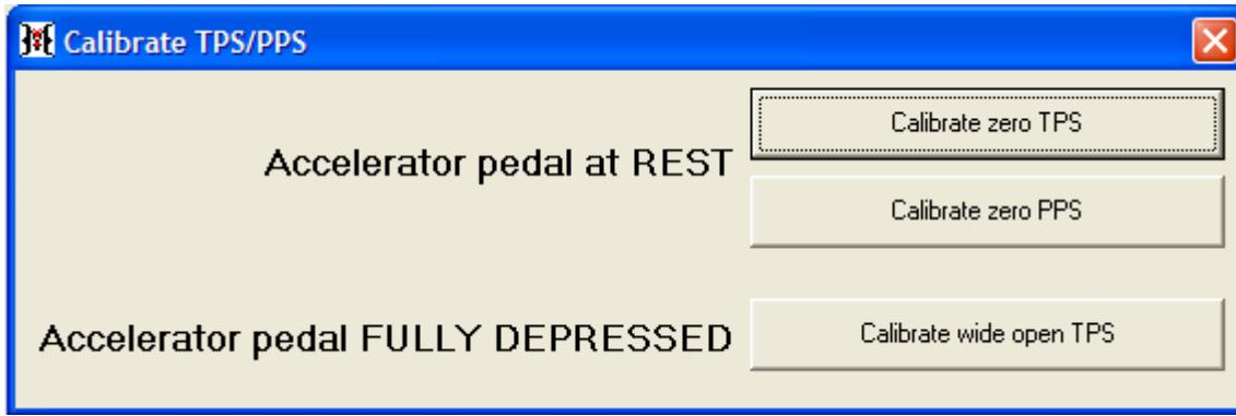
With your foot off the accelerator pedal, click the **Calibrate zero TPS** and **Calibrate zero PPS** buttons. Then, push the accelerator pedal as far as you are able to and, while holding it in that position, click the **Calibrate wide open TPS** button.
